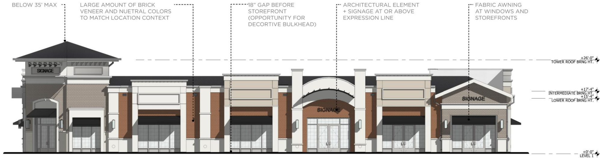
MATERIAL CHOICES AND ARCHITECTURAL ELEMENTS PER DESIGN GUIDELINES (ELEVATION 'B' SHOWN FOR REFERENCE)
