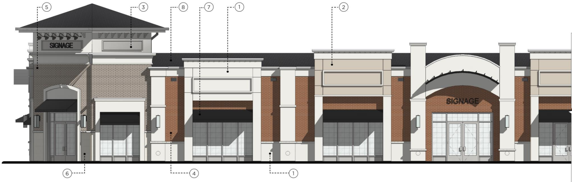
ENLARGED BUILDING ELEVATION - CORNER DESIGN AND MATERIALS
