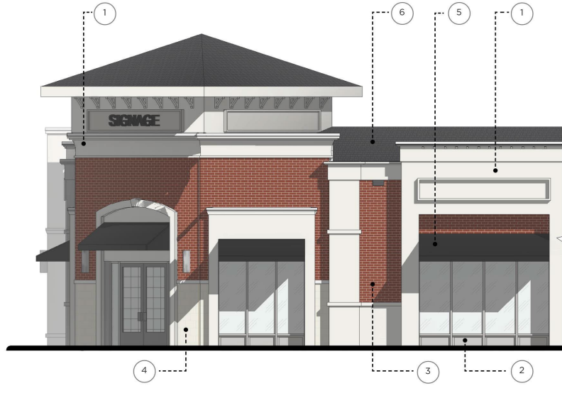
ENLARGED BUILDING ELEVATION - CORNER DESIGN AND MATERIALS
