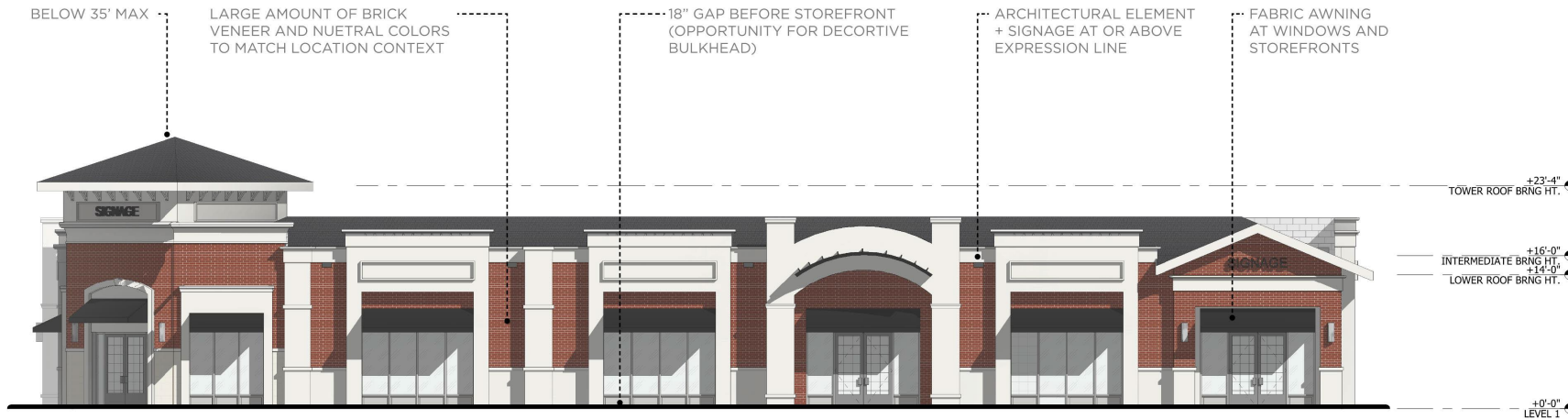
MATERIAL CHOICES AND ARCHITECTURAL ELEMENTS PER DESIGN GUIDELINES (ELEVATION 'B' SHOWN FOR REFERENCE)
