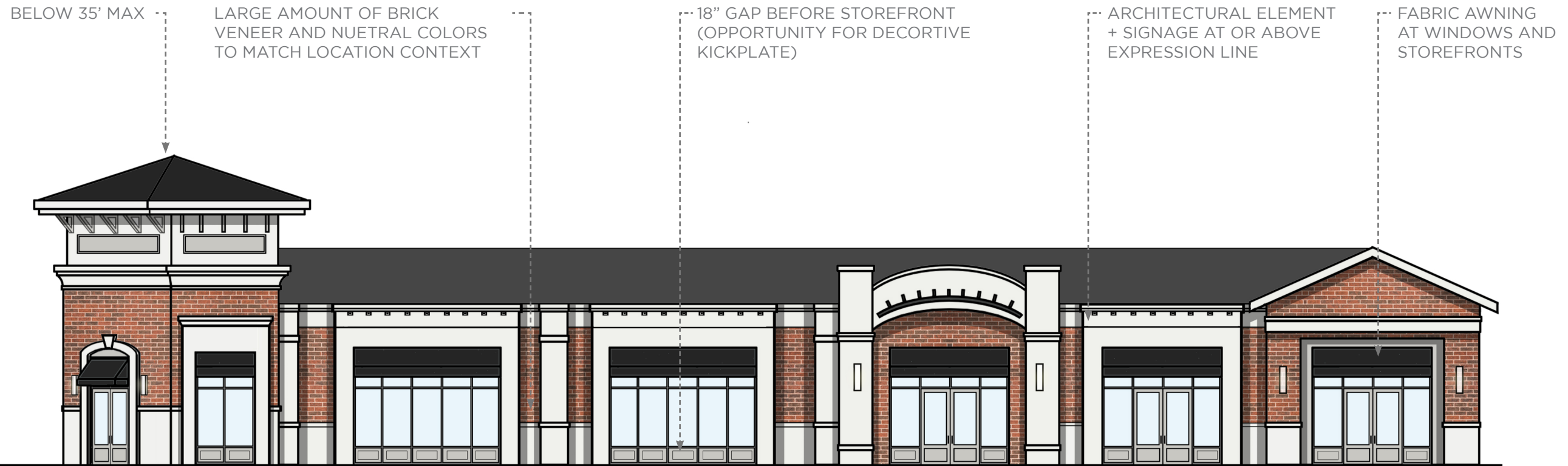
MATERIAL CHOICES AND ARCHITECTURAL ELEMENTS PER DESIGN GUIDELINES (ELEVATION 'A' SHOWN FOR REFERENCE)
