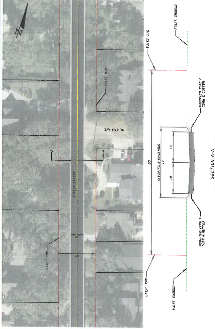
Inverted Crown Paved Road with Inlets – Minimal Clearing of Right of Way
