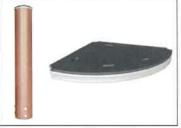
ELEMENTS decks are made of 17.8mm thick HPL supported by a unique designed aluminium frame with multiple attachment options by usage of aluminium connectors. The main posts are made of high quality pre-galvanized steel with powder coated top finish. Post tops are closed with caps of UV stabilized nylon (PA6).
