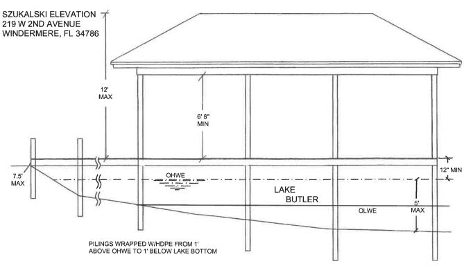
MIN DEPTH OF 2' BELOW THE MEAN ANNUAL LOW WATER ELEVATION IN THE SLIP AREA
